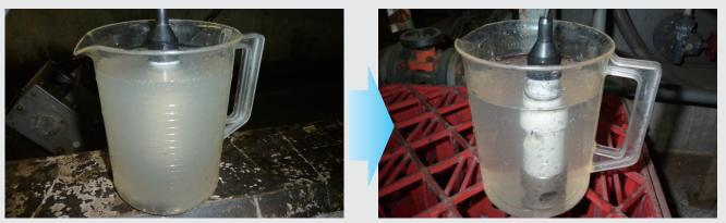
\*The treated water in the photo is not a supernatant (the top clear layer of liquid above solid residue after precipitation, etc.). It is water extracted during aeration stirring. A key characteristic of Aquablaster is that it even treats suspended solids. Please feel free to tour a facility in operation. (\*No activated sludge used)
