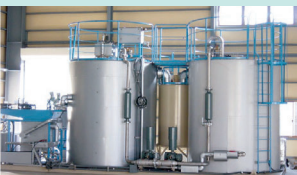
■ Nikko Co., Ltd. 10m 3 /day Industrial wastewater treatment facility Succeeded in stable treatment of wastewater with high load and high fluctuation
